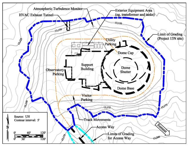
Figure 2-7: TMT Observatory Plan View and Grading Plan
