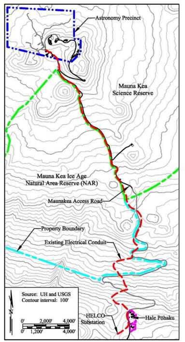
Figure 2-10: Route of Electrical Conduit
