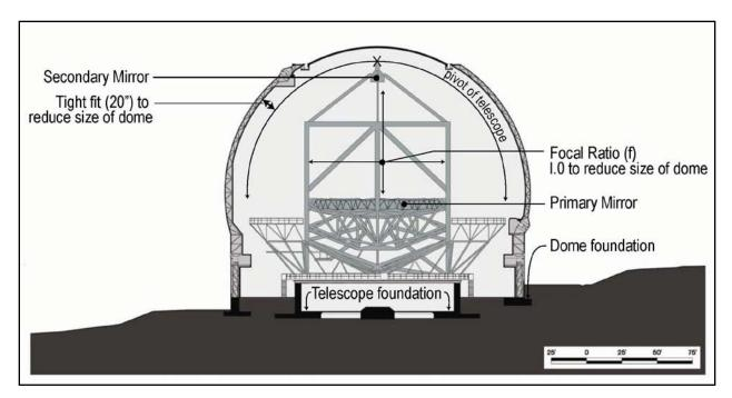
Figure 3-25: Overview of TMT and Dome Design
