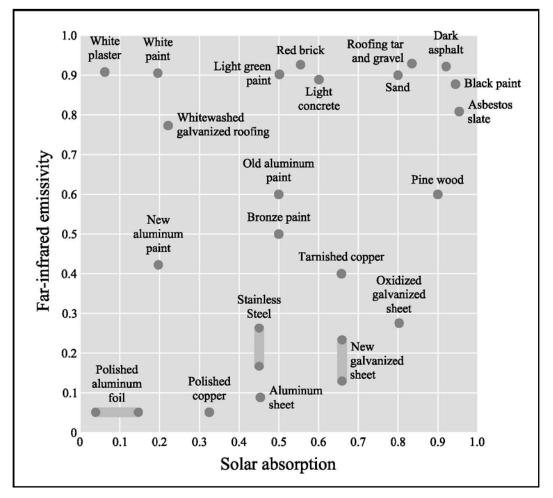
Figure 3-9: Finish Emissivity and Absorption
